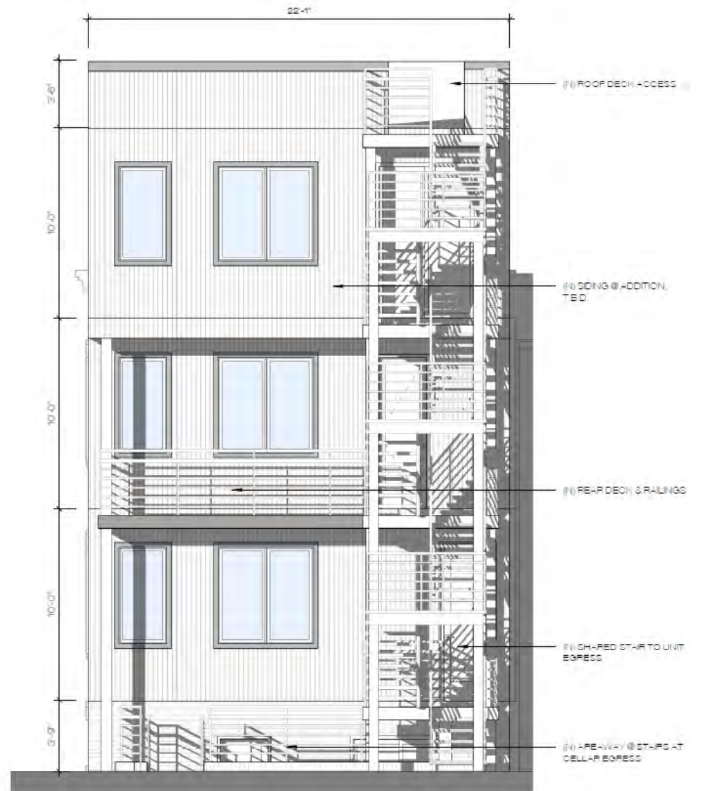
② ELEVATION - SOUTH (REAR) 3/16" = 1'-0"
